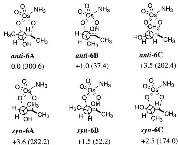
**Figure 7.** Transition structures for the osmylation of (*Z*)-3-penten-2-ol with relative energies (kcal/mol) and dihedral angles O—C—C=C.
